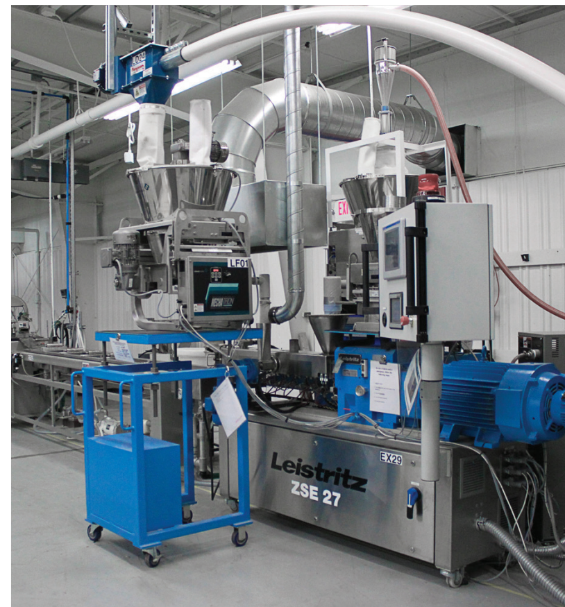
Teel does some of its own compounding, and produces proprietary formulations for others, on this Leistriz 27-mm corotating twin.
