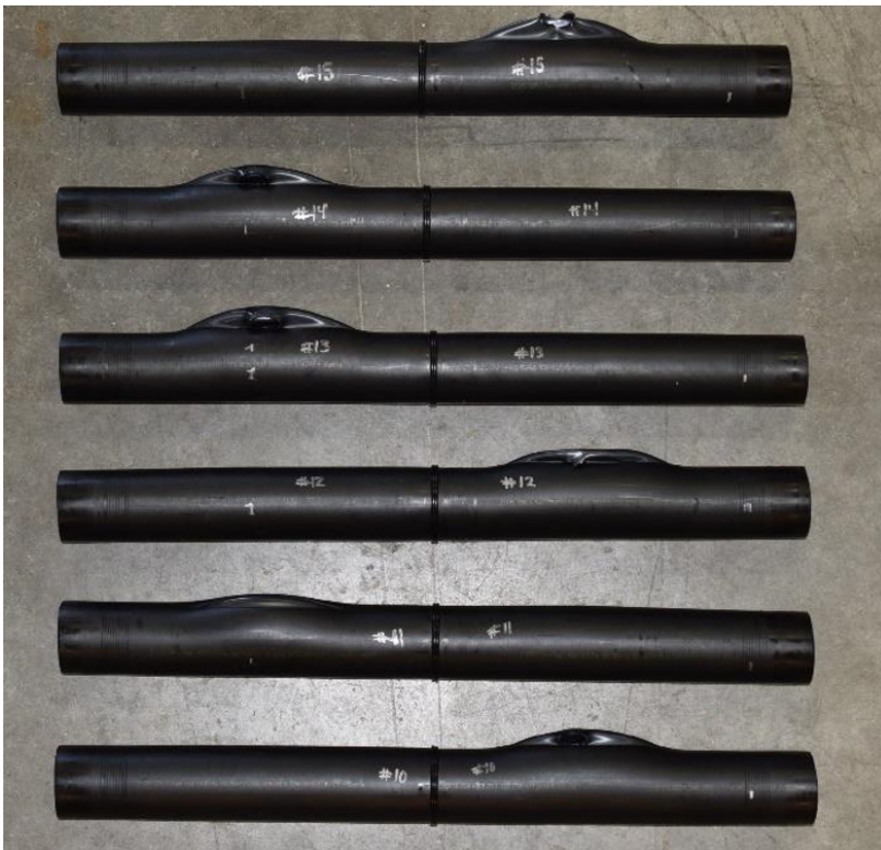
Figure 10: Teel's 2710 and 2708 quick burst test samples after testing
