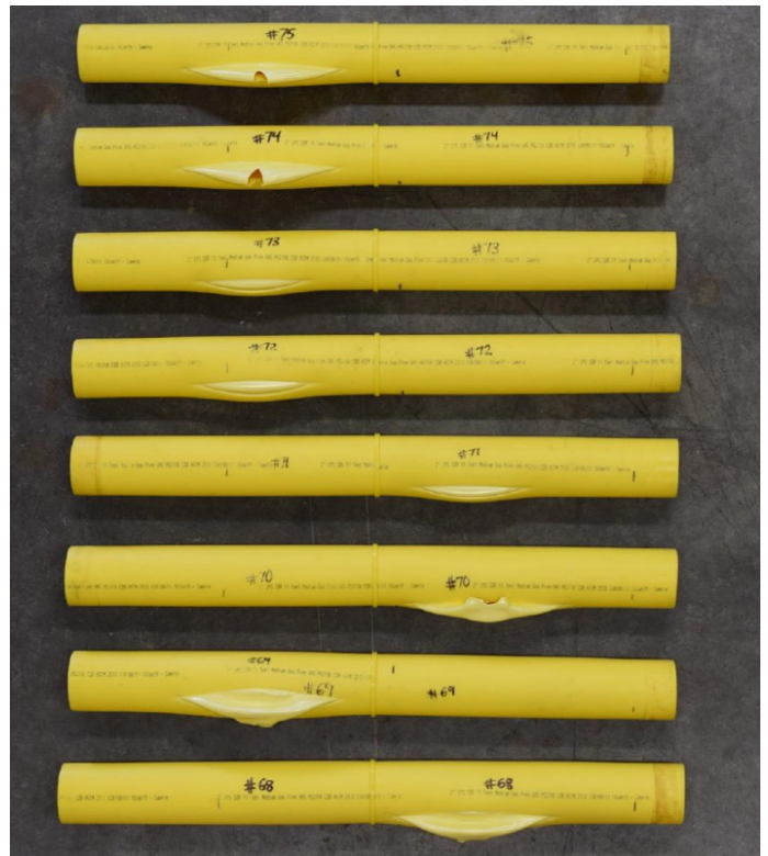
Figure 10: Teel's 2710 and 2708 quick burst test samples after testing
