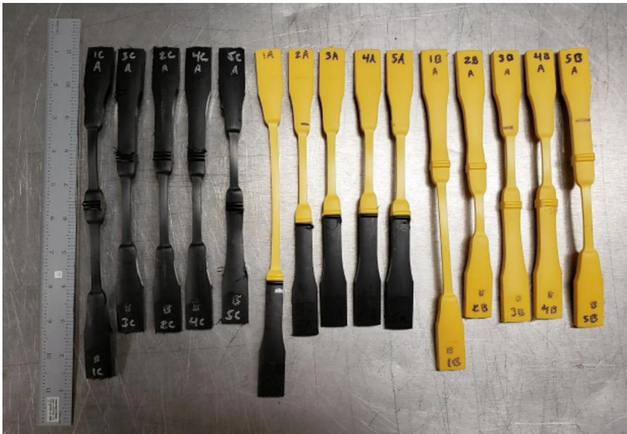
Figure 7: Teel's tensile properties test samples before and after testing
